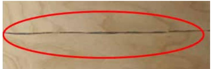
Since wood has natural defects (such as knots, cracks, general wood bruising and small holes), large defects that might compromise performance are removed during material production. The PET carrier remains constant and untorn. There can be up to 140 wood separations in a 5000 ft roll (the average is approx. 70 wood separations or fewer).
