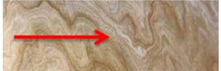
A tape splice is a section of the face material where both the wood and the PET carrier have been cut to remove defects and then taped together on the backside of the carrier with a thin transparent tape. The maximum number of splices per 5000 ft roll is 10.
